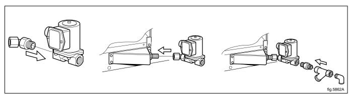
Mount the hose with wires between steam valve and machine.
