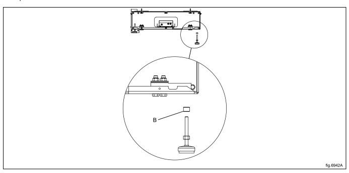
Lift the machine and remove the transport pallet.
