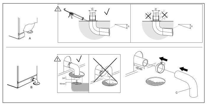
We strongly recommend to drain under the machine for hygiene and safety reasons. Make sure the drain connection is tight. Otherwise the warm steam from the drainage water can damage the components.
