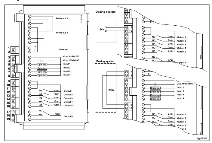
Signals for external liquid supplies 6-10 are connected to the terminal block 6–10 located next to the I/O board where terminal:
