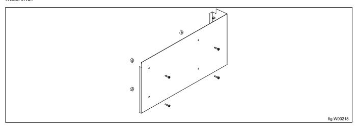
The screws on the side panels (A) shall not be tightened all the way in.
