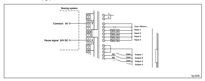
Connection 7. If this is connected, an error message will be displayed if any of the chemical tanks are empty. The program will continue, however.
