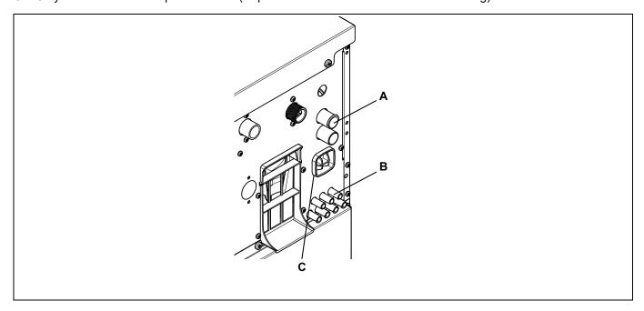
Always connect hoses on connections A with a hose clamp.
