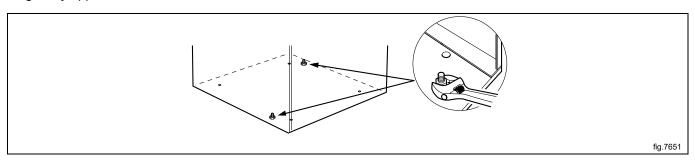
Remove the machine from the pallet.
